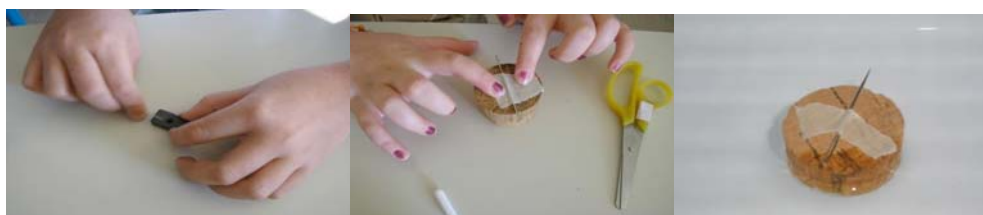
Figure 4. Building a rudimentary compass
